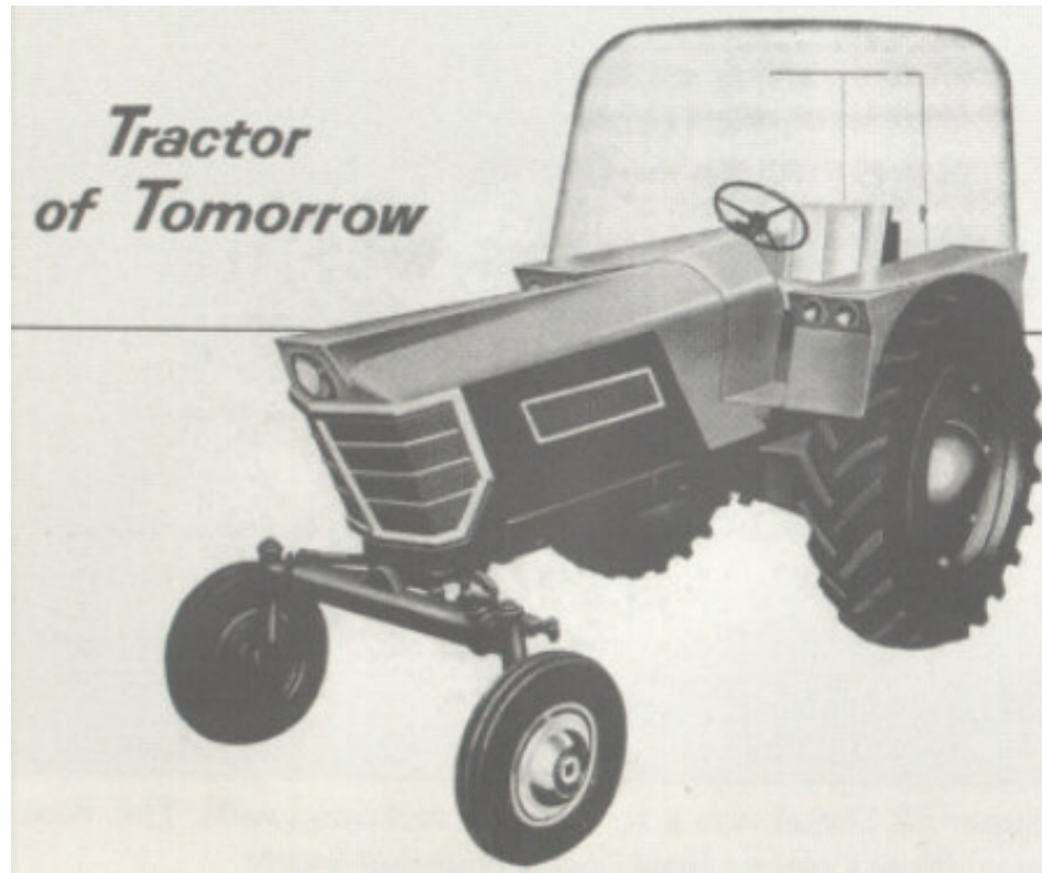
1960 Oliver future tractor (bubble cab, retractable ladder, auto gate opener)
